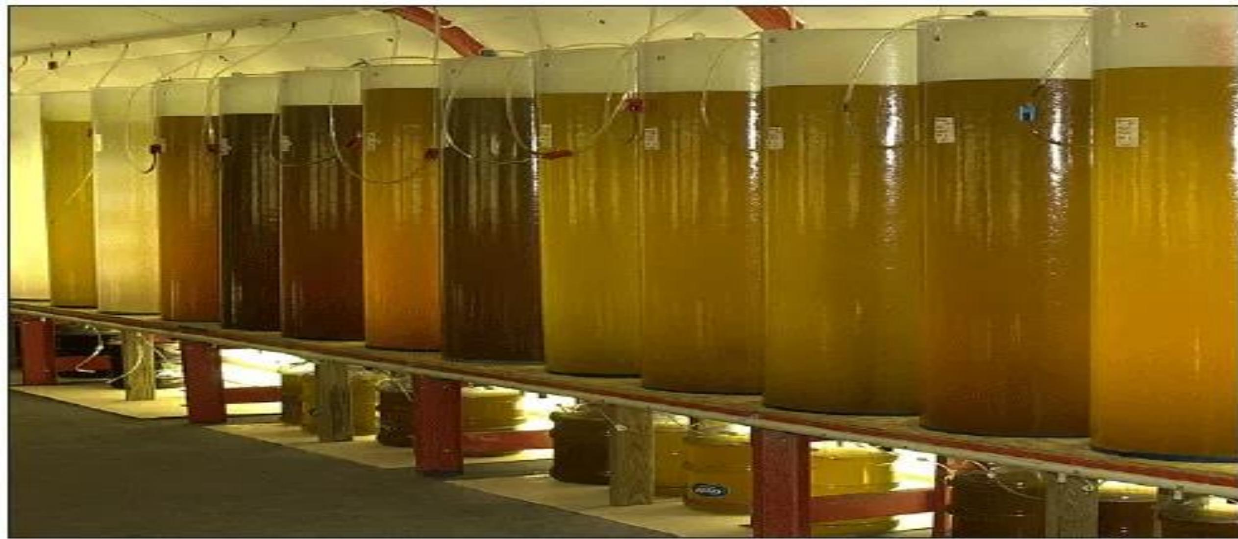
**Translucent fiberglass cylinders (200-L) are commonly used for production of microalgae up to harvest and feeding. For large-scale algae production, they can be used to inoculate 2,000- to 5,000-L mass culture tanks.**
